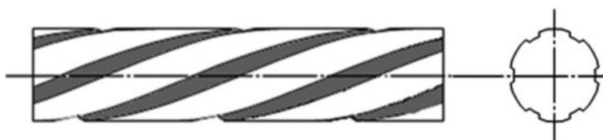
Figure 1 Example of shape and cross-section of steel bars
